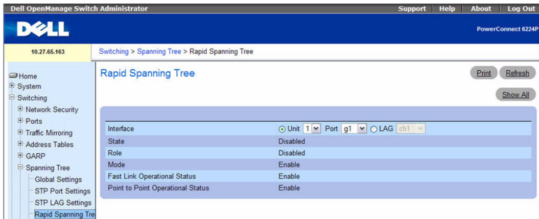
Figure 7-43. Rapid Spanning Tree
